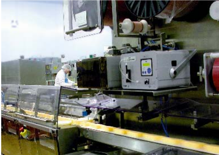
Gas mixer-analyser combination in a cheese packaging facility
