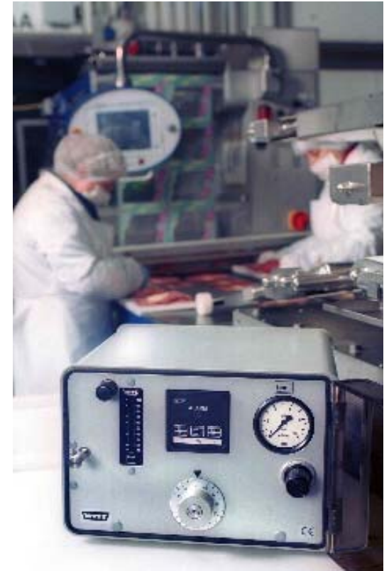
Individual gas mixtures for 17 lines of a big meat packer
